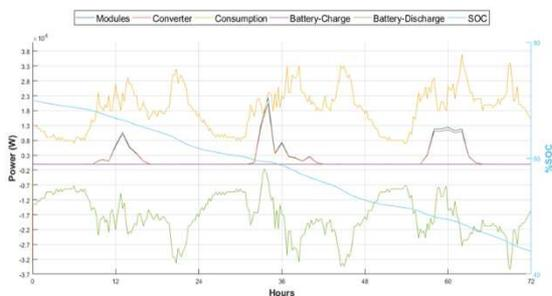
Figure 13. Power generation SOC present in the system in the LOWEST scenario.
