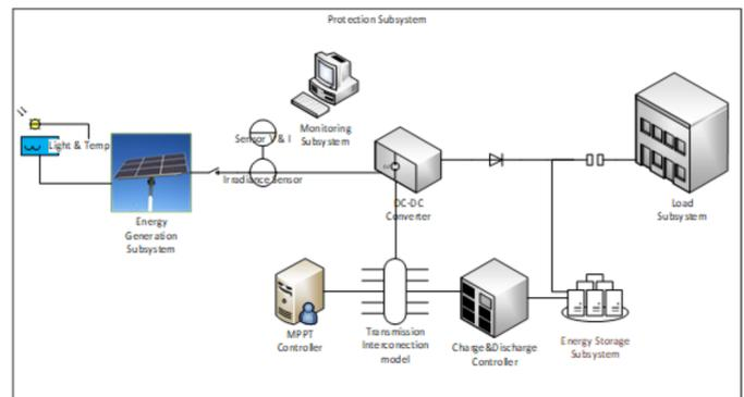
Figure 1. Microgrid diagram.
