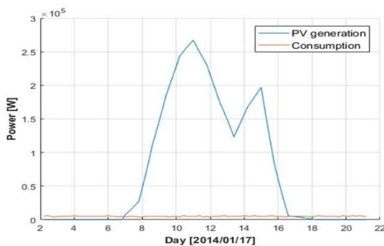
Figure 4a. Solar PV potential versus time consumption of the building in a summer day.
