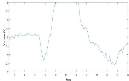
Figure 8. Supply voltage to the building in the system for WINTER scenario.
