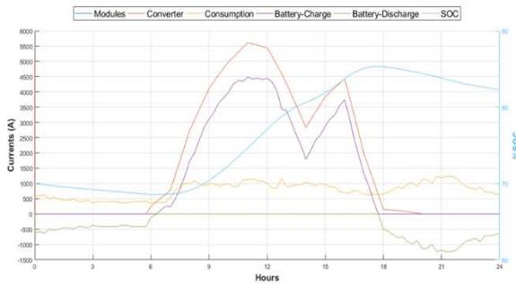
Figure 11. Currents flows & SOC present in the system for the SUMMER\* scenario.
