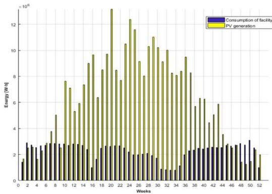
Figure 6. Solar PV potential versus consumption of the building
