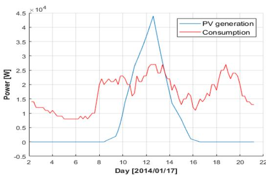
Figure 4b. Solar PV potential versus time consumption of the building in a winter day.
