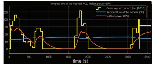
Fig. 8: Gas boiler power profile for a 1 hour simulated consumption profile.
